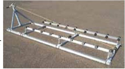
10' long ramp with roller bunks, keel rollers, winch and rope.
